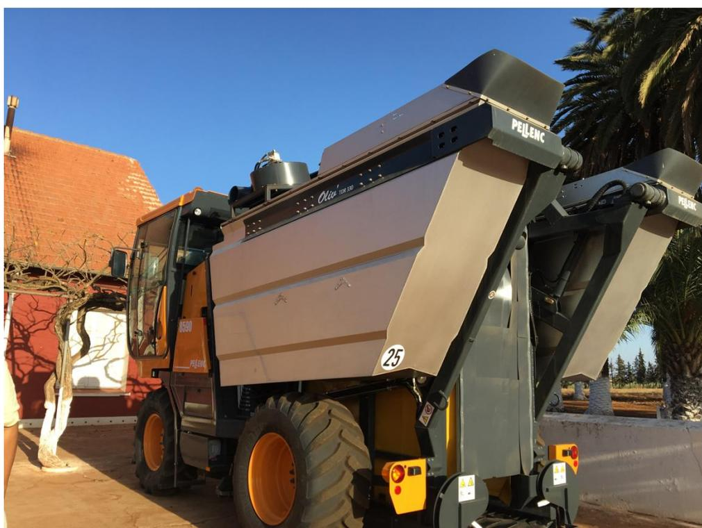
*Figure 3: Pellenc 8590, is owned by an olive farm in the region of the Saïs. The machine can harvest up to 1ha per hour (around 16ha per day) while at the same time separating the fruits from the wood so that one can skip a step at the factory. It can also be used for applying phytosanitary treatments or any leaf or air straying treatment, and can cover up to 40ha per day (Photography taken by C. Gharios 2017)*
